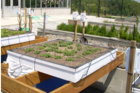
Figure2. Experimental greenroof platform constructed as part of this project
