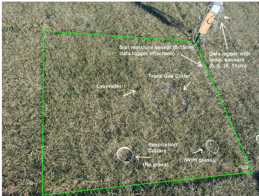
Figure 7. An instrumented sampling unit. Each unit has two respiration collars, one with vegetation and one with vegetation removed; one trace gas collar, and one tension lysimeters installed at 30cm. Each split also has data loggers collecting soil temperatures at the soil surface, 5, 10, and 15cm, and soil moisture at 5-15cm.
